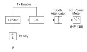
Figure 3.1 T838/839 Test Equipment Set-up
